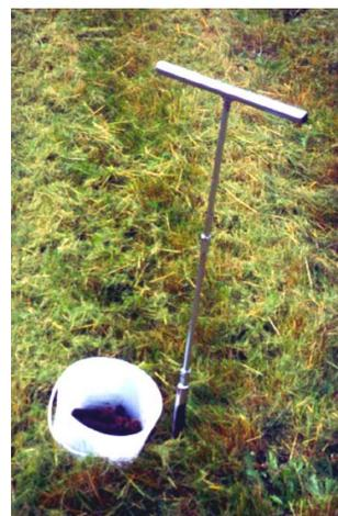
**Figure 4.** Soil probe
