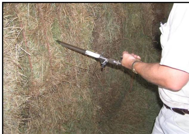
Figure 2. Collecting a core from a square bale
