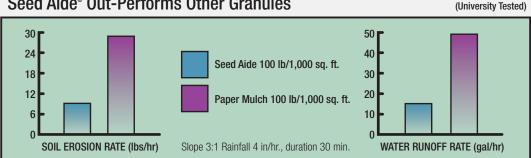
At comparable application rate of 100 lbs per 1000 sq ft, Seed Aide reduced soil erosion by 68.9% and water runoff by more than 63.2% versus the competitor's paper pallets.
